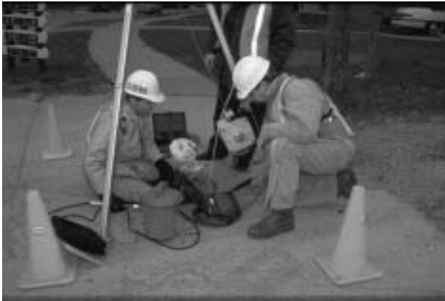
Ben Sherman and Mark TenBroek of CDM evaluate flow conditions in southwest Detroit as part of the Greater Detroit Regional Sewer System Combined Sewer Overflow (CSO) modeling work.
